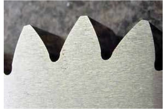
Figure 1: Asymmetric gear with tooth root generated with protuberance hob.
